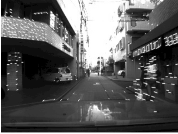
Fig. 6. Flow vector calculation in driver's view
