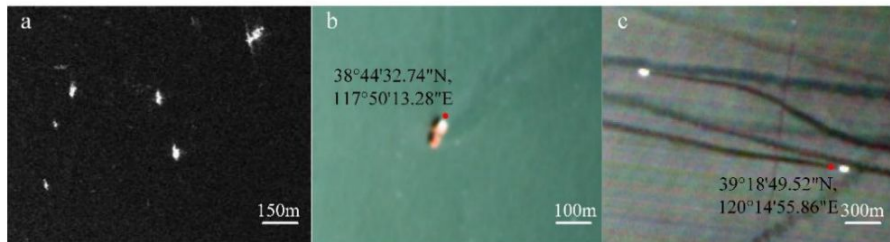
Figure 1. (a) The SAR image with the resolution of 15 m in SSDD dataset [31], The (b) true color image of 460–520 nm, 520–600 nm and 630–690 nm with resolution of 10 m in 38°44′32.74″N,117°50′13.28″ from SDGSAT-1 multispectral imager, and (c) pseudo-color image of 8~10.5 \mu m, 10.3~11.3 \mu m 11.5~12.5 \mu m with resolution of 30 m in 39°18′49.52″N,120°14′55.86″E from SDGSAT-1 TIS.
